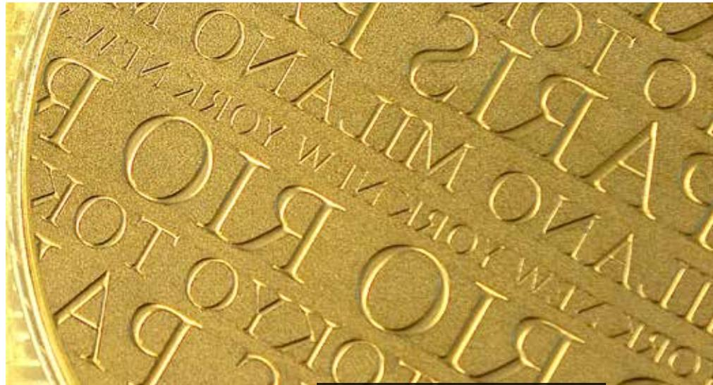
Kurz will showcase what it calls Digital Metal where the metallic film is applied to an area printed by dry or liquid toner which it adheres to.
